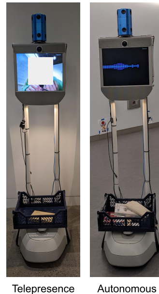
Fig. 2: The two study conditions. Both robots are equipped with a basket of items for delivery. The telepresence robot is shown on the left with the operator’s face on the screen. The perceived autonomous robot shows an example of the sound visualization mid-speech.
