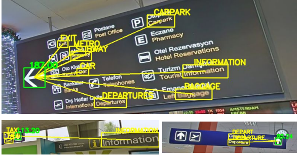
Figure 6. Several examples of output images from our vision system. Bounding boxes for text are in yellow, bounding boxes for arrows are in green. Lines illustrate groupings of text with respective arrows, and the number value is the angle orientation of the detected arrow.
