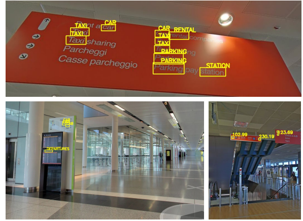
Figure 7. A selection of failure case outputs from our perception system. Failures often occur when text and arrows are very small relative to sign size. Text and bounding boxes are in yellow.
